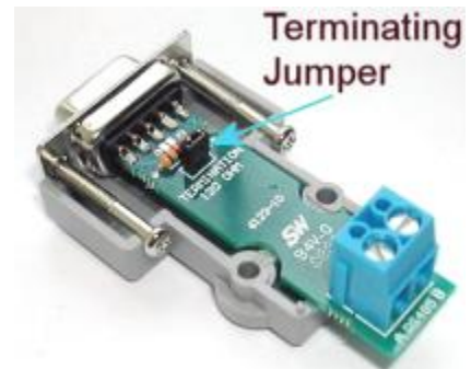
Fig 3-19 RS485 120 Ohm Jumper
